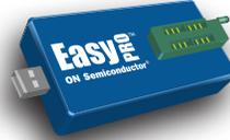
EasyPRO™ is a user-friendly, portable programming tool for ON Semiconductor serial EEPROMs (I<sup>2</sup>C, SPI, Microwire)
