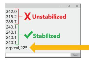
Once the readings have stabilized, issue the calibration command. In this case orp:cal,225
