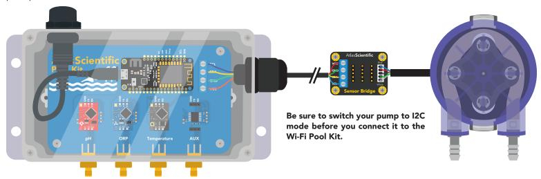
You can directly connect an EZO Pump to the Wi-Fi Pool Kit without the sensor bridge however you must remove the data cable connector and manually put the pump into I2C mode.
