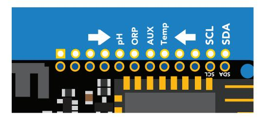
The first three pins (pH, ORP and Aux) must be set low to power on the sensor. The last pin (Temp) must be set high to power on the sensor.
