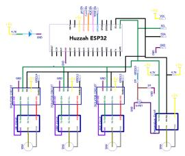
Each of the four main sensor ports have an enable pin, which must be set correctly to power the sensor. The enable pins are found here:
