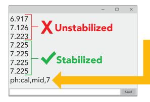
Once the readings have stabilized, issue the Mid point calibration command. ph:cal,mid,7
