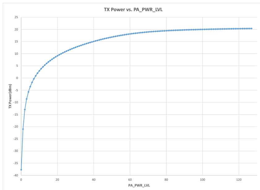
Figure 8. +20 dBm TX Power vs. PA\_PWR\_LVL
