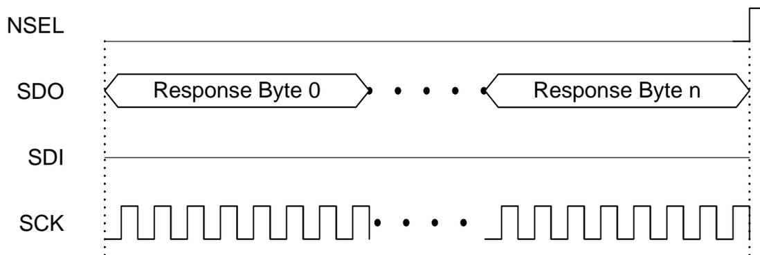
Figure 4. SPI Read Command—Clock Out Read Data
