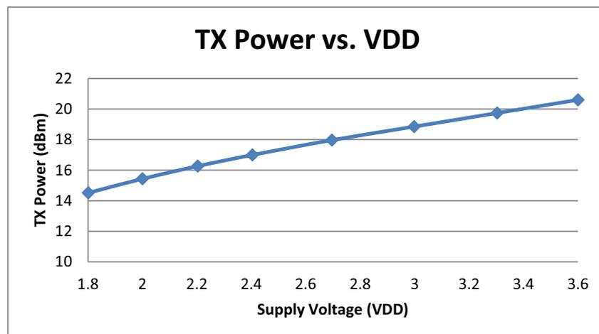
Figure 9. +20 dBm TX Power vs. VDD
