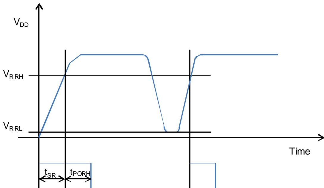
Figure 6. POR Timing Diagram
