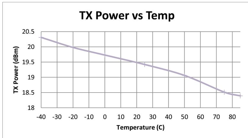
Figure 10. +20 dBm TX Power vs. Temp
