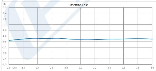
Click the following link (or enter part number in "SEARCH" on website) to obtain additional part information including price, inventory and certifications: High Power Circulator with 18 dB Isolation from 2 GHz to 4 GHz, 100 Watts and SMA Female PE83CR1030
