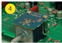
Mount the volume unit to the main PCB of TU-8600/TU-8600R, and mount the whole unit to the chassis.
