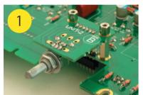
Remove the currently mounted volume pot with PCB from TÚ-8600/TU-8600R.
