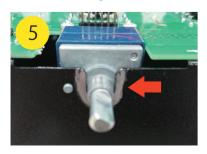
In order to connect the volume shaft with the chassis ground, trim the chassis paint of the chassis surface and fix the volume with the nut. Without this process, a hum noise occurs when you touch the volume knob.
