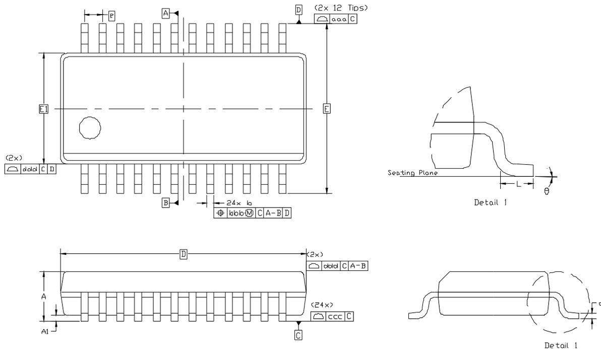
Figure 3. 24-Pin SSOP
