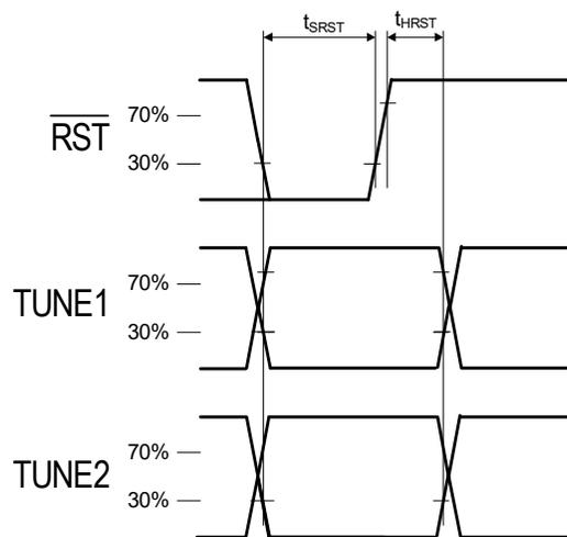
**Figure 1. Reset Timing**
