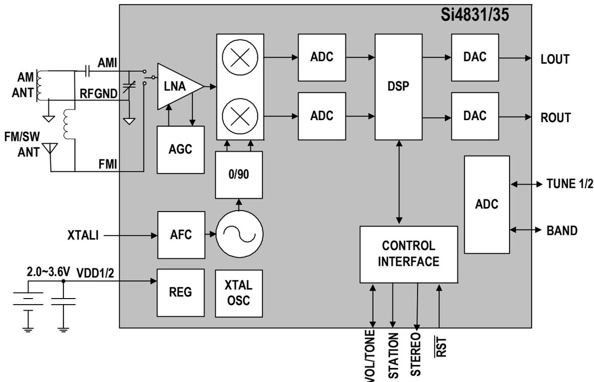
Figure 2. Si4831/35-B30 Functional Block Diagram
