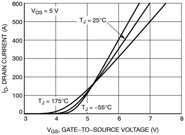
Figure 2. Transfer Characteristics
