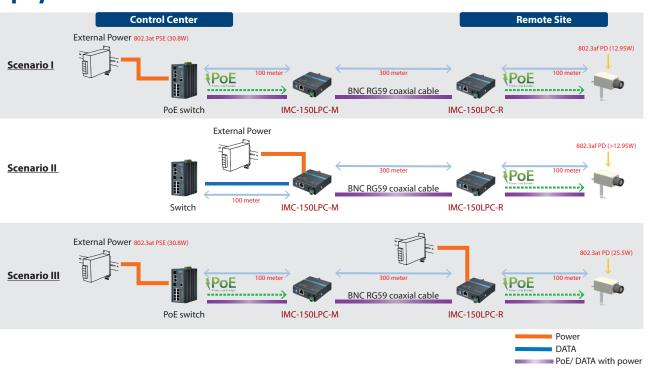
Note1: Advantech uses RG59 coaxial cables of Belden's 551945 010100, with the DCR conductor resistance value of 15 Ohm/1000ft to conduct tests. The transmitted output power and distance depends on resistance value of coaxial cables installed at field sites.
