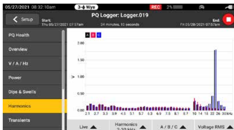
A full range of harmonics are available from the first 50 integer harmonics and from 2 kHz to 30 kHz
