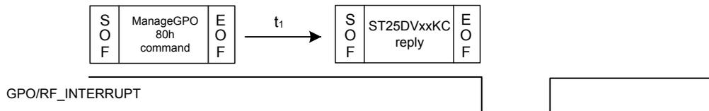
2) VCD sends a ManageGPO command (any value) and ST25DVxxKC replies with error. GPO/RF\_INTERRUPT remains high-Z.
