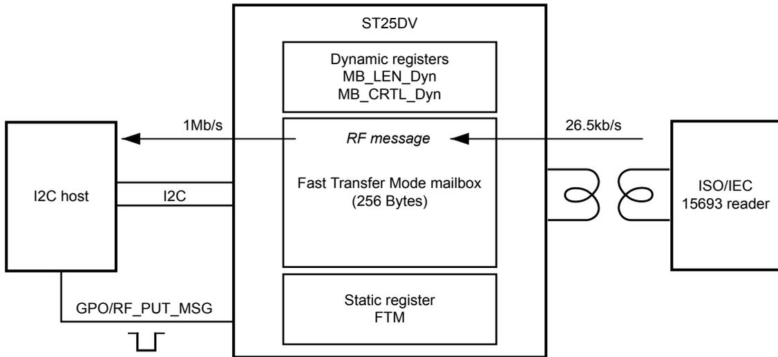
To send data from the I<sup>2</sup>C host to the RF reader, fast transfer mode must be enabled, the mailbox must be free, V<sub>CC</sub> power must be present, and the I<sup>2</sup>C host must first write the message containing data in the mailbox.
