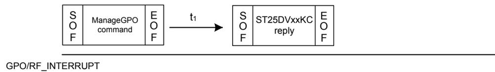
3) VCD sends a ManageGPO command (any value) and ST25DVxxKC stays quiet (command not for this VICC, or quiet state). GPO/RF\_INTERRUPT remains high-Z.
