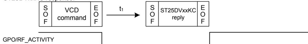
2) VCD sends a write command and ST25DVxxKC replies after write completed. GPO/RF\_ACTIVITY is released after ST25DVxxKC response.
