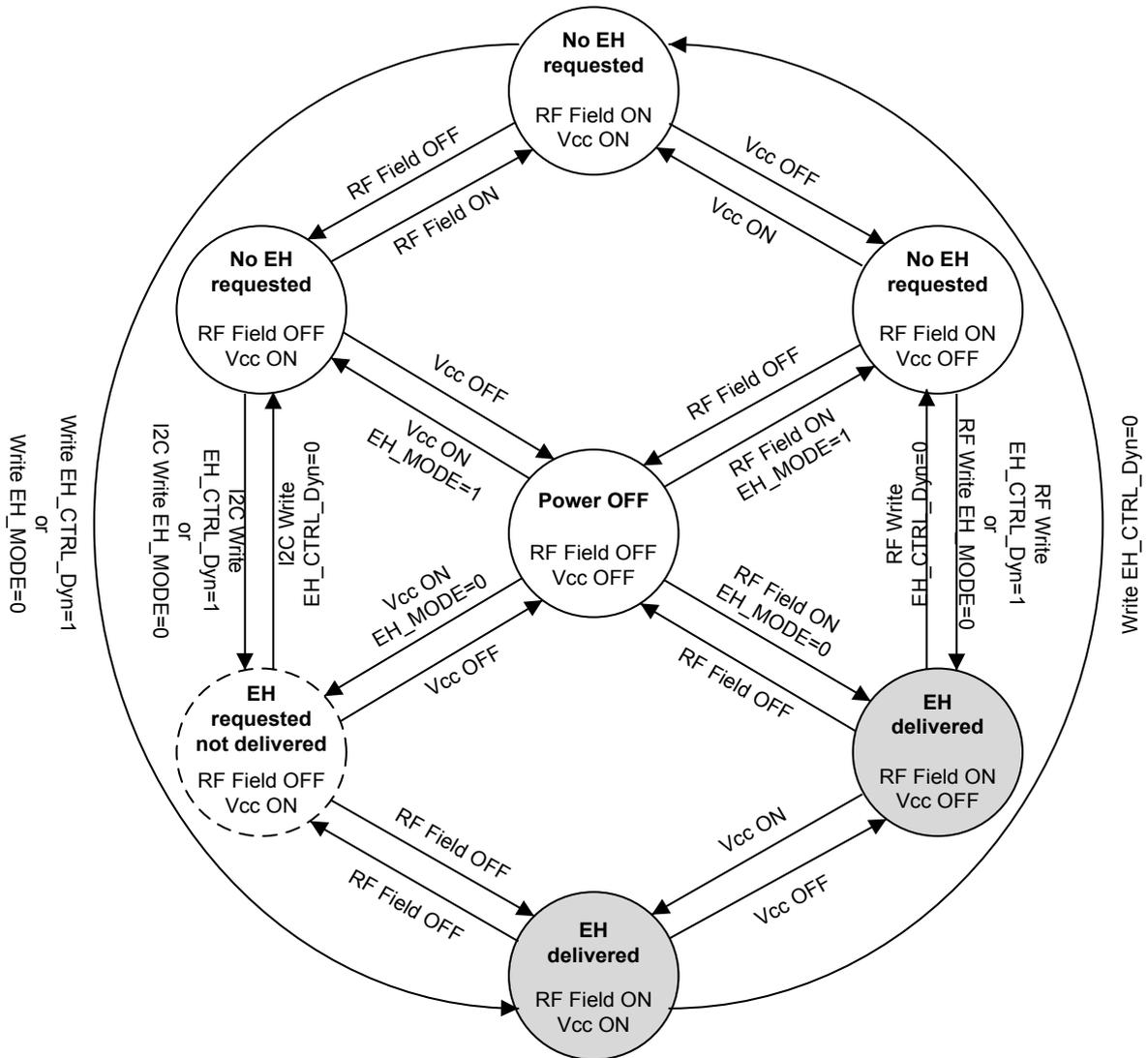
**Note:** Power is delivered on V<sub>EH</sub> only if harvested energy is sufficient to supply ST25DVxxKC and leave over power. Grey color indicates the states where power is delivered on V<sub>EH</sub> pin.
