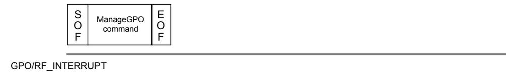
4) VCD sends any command other than ManageGPO command and ST25DVxxKC replies. GPO/RF\_INTERRUPT remains high-Z.
