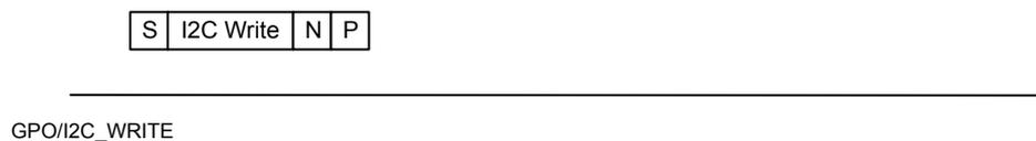
3) I2C host sends a valid write command to Dynamic register or Mailbox. ST25DVxxKC program the data with no programming cycle. GPO/I2C\_WRITE remains high-Z.
