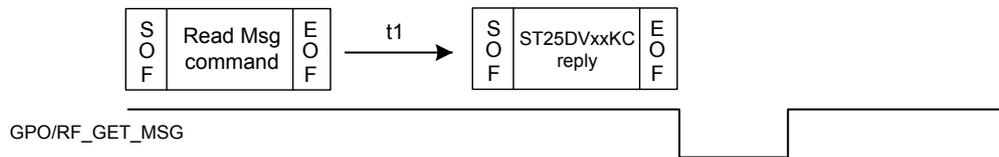
2) VCD sends a Read Message or Fast Read Message command and ST25DVxxKC replies with error. GPO/RF\_GET\_MSG remains high-Z.
