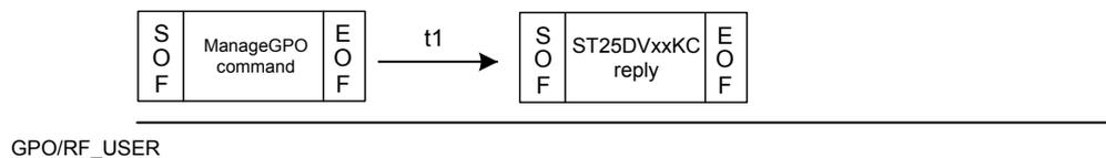
4) VCD sends a ManageGPO command (any value) and ST25DVxxKC stays quiet (command not for this VICC, or quiet state). GPO/RF\_USER remains high-Z.
