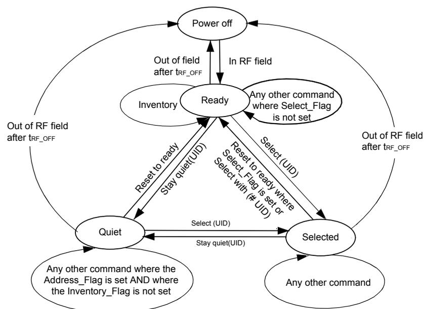
1. The ST25DVxxKC returns to the Power Off state if the tag is out of the RF field for at least  $t_{RF\_OFF}$ . The intention of the state transition method is that only one ST25DVxxKC should be in the Selected state at a time.
