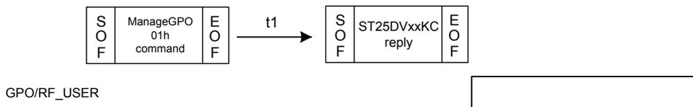
3) VCD sends a ManageGPO command (any value) and ST25DVxxKC replies with error. GPO/RF\_USER remains high-Z.
