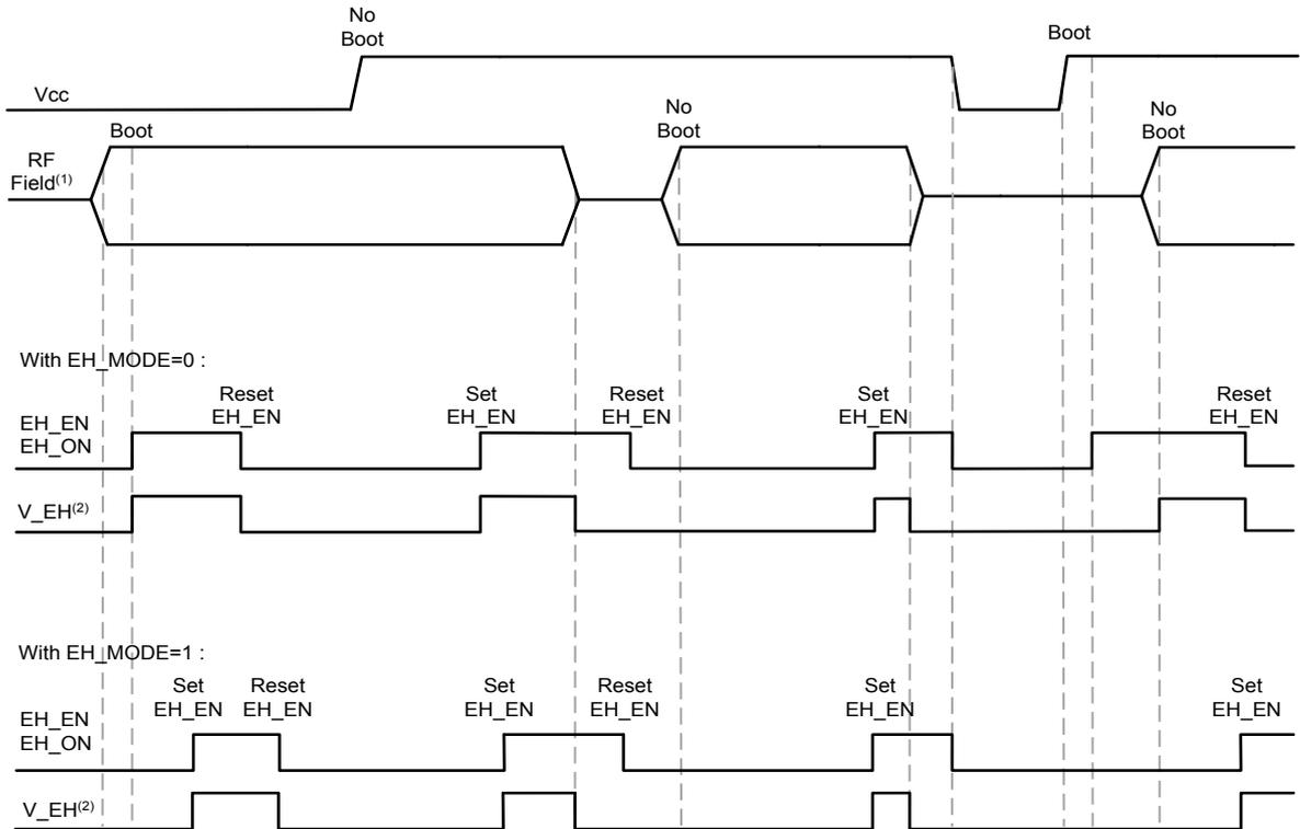
1. We suppose that the captured RF power is sufficient to trig EH delivery.
