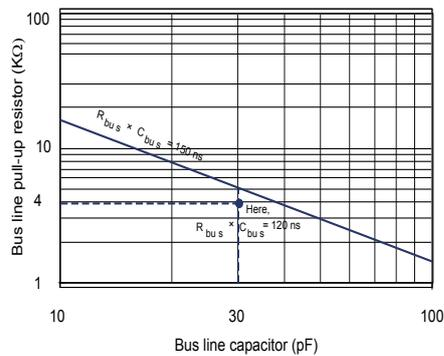
The  $R_{bus} \times C_{bus}$  time constant must be below 150 ns. The time constant line is represented on the left.
