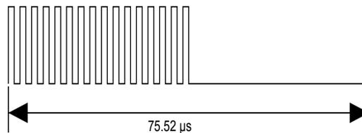
For the Fast commands, a logic 1 starts with an unmodulated time of 37.76  $\mu\text{s}$  followed by 16 pulses at 423.75 kHz ( $f_C/32$ ), as shown in Figure 92.
