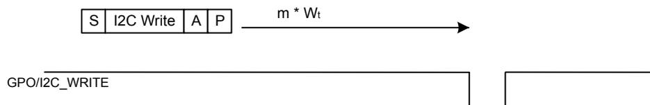
2) I2C host sends an invalid write command to EEPROM. ST25DVxxKC does not program the data into EEPROM. GPO/I2C\_WRITE remains High-Z.
