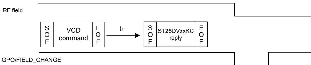
3) RF field disappears and ST25DVxxKC is not powered through VCC. GPO/FIELD\_CHANGE doesn't generate any pulse.
