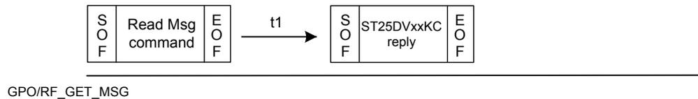
3) VCD sends Read Message or Fast Read Message command and ST25DVxxKC stays quiet (command not for this VICC, or quiet state). GPO/RF\_GET\_MSG stays high-Z.
