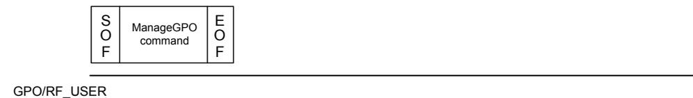
5) VCD sends any command other than ManageGPO command and ST25DVxxKC replies. GPO/RF\_USER remains high-Z.
