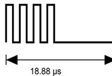
For the Fast commands, a logic 1 starts with an unmodulated time of 9.44  $\mu\text{s}$  followed by four pulses of 423.75 kHz ( $f_C/32$ ), as shown in Figure 90.
