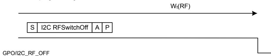
3) I2C host sends a valid I2C RFSwitchOff command and I2C\_RF\_SWITCHOFF\_EN = 0. RF is not switched off and the GPO/I2C\_RF\_OFF remains high-Z.
