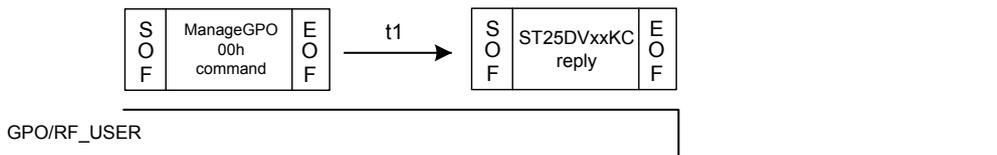
2) VCD sends a ManageGPO command with value 01h (reset GPO) and ST25DVxxKC replies. GPO/RF\_USER is set high-Z low after ST25DVxxKC response.
