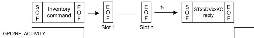
5) VCD sends a command and ST25DVxxKC stays quiet (Stay Quiet command, command not for this VICC, or quiet state). GPO/RF\_ACTIVITY remains high-Z.
