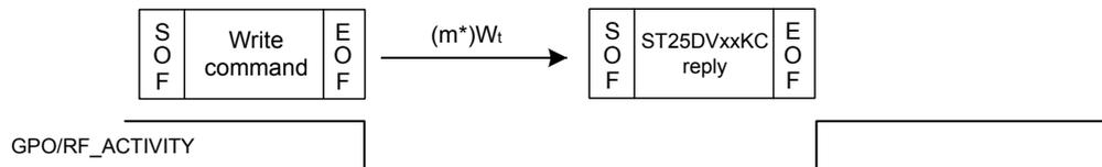
3) VCD sends a write command with option flag set to 1, and ST25DVxxKC replies after receiving EOF. GPO/RF\_ACTIVITY is released after ST25DVxxKC response.
