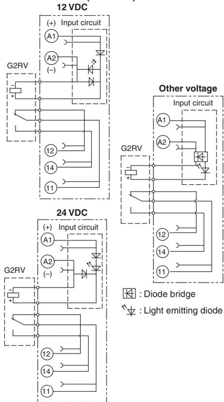
**Models with latching lever (with test switch)**
