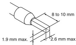
3. If you use AWG24 to AWG22 (0.25 to 0.34 mm<sup>2</sup>) wires, UL certification will not apply.
