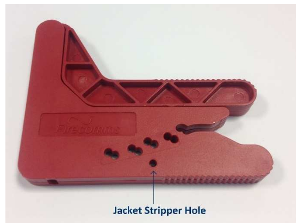
Figure 6. Jacket Stripper on POF cutter
