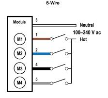
1 = Brown 2 = Blue3 = White 4 = Black 5 = Gray 6 = Red7 = Yellow M1 = Module 1 M2 = Module 2 M3 = Module 3 M4 = Module 4 M5 = Module 5 M6 = Module 6
