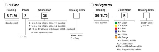
Select the 5-pin/wire base for tower light configurations of up to 4 modules. Select the 7-wire base for tower light configurations of up to 6 modules.
