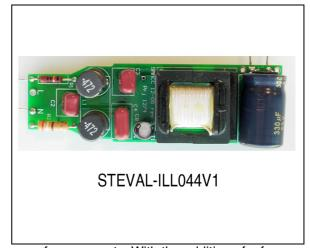
use of components. With the addition of a few extra components the HVLED815PF is made to draw near-sinusoidal input current from the AC line. The circuit regulates LED current over a wide range of line voltage and LED string voltage, and is dimmable with standard Triac-based dimmers.
