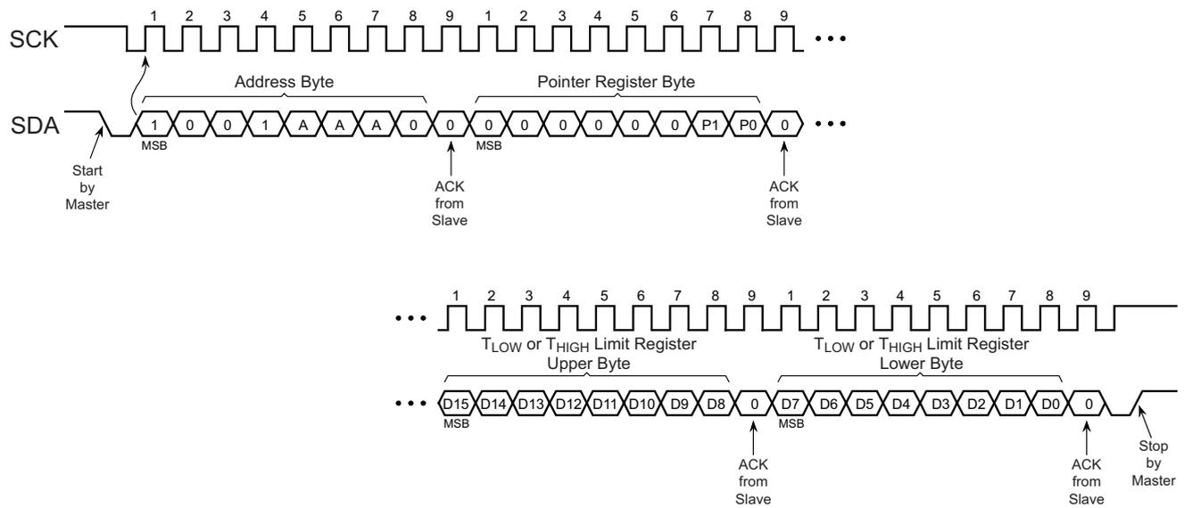
**Figure 5-7. Read from  $T_{LOW}$  or  $T_{HIGH}$  Limit Register**
