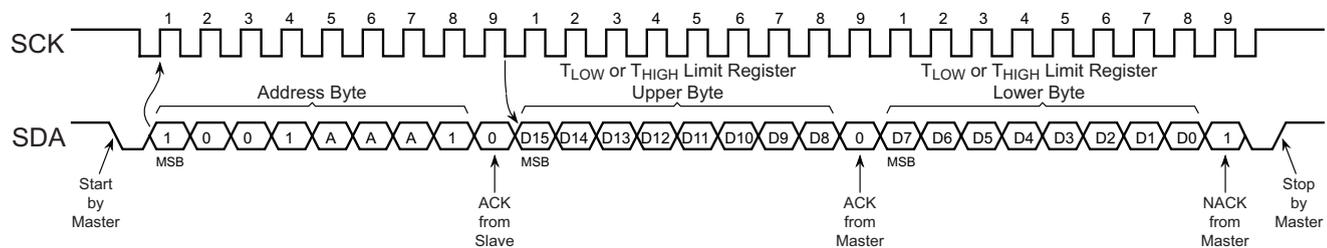
Note: Assumes the Pointer Register was previously set to point to the  $T_{LOW}$  or  $T_{HIGH}$  Limit Register.
