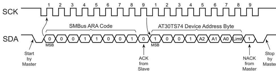
Note: The Limit bit (the LSB) of the device address byte will be one or zero depending on if the T<sub>HIGH</sub> or T<sub>LOW</sub> limit was exceeded.
