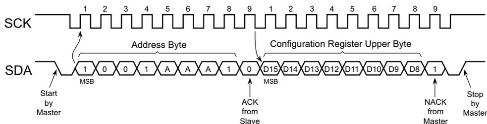
Note: Assumes the Pointer Register was previously set to point to the Configuration Register.
