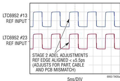
**Step 2: ParallelSync Multichip Clock Alignment**
