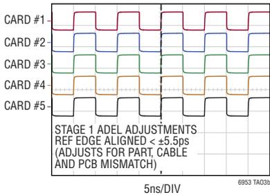
**Step 2: ParallelSync Multichip Clock Alignment**
