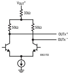
Figure 3. Simplified CML Interface Schematic (All OUTx)
