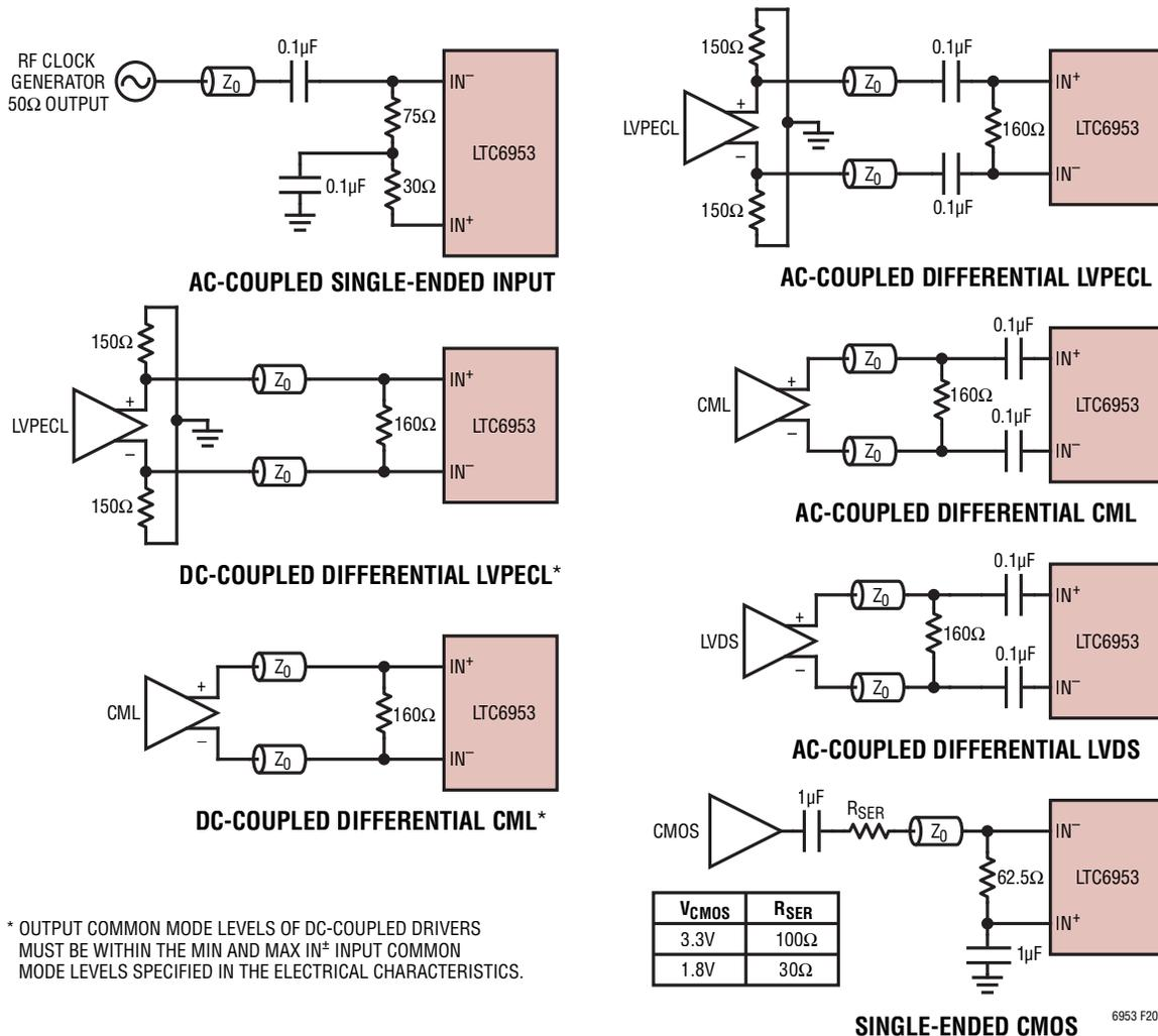
Figure 20. Common Input Interface Configurations. All Z<sub>0</sub> Signal Traces Are 50Ω Transmission Lines
