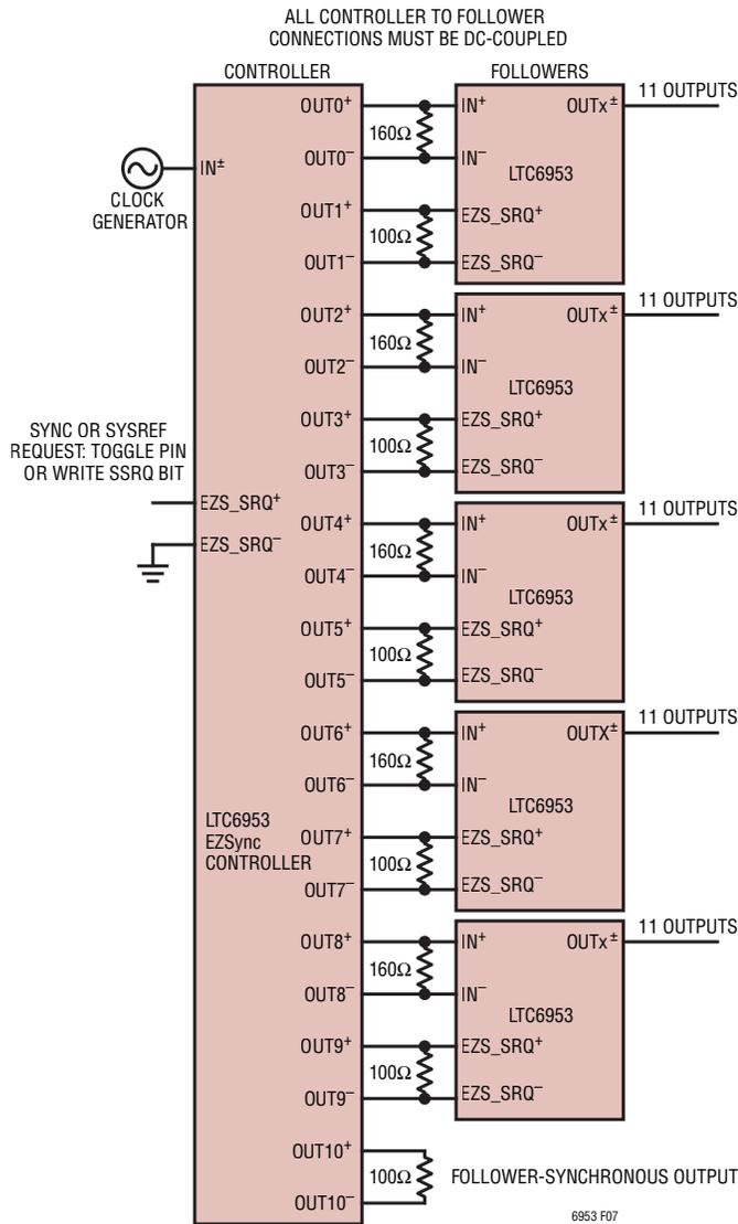
**Figure 7. EZSync Multichip Synchronization with Request Pass-Through**
