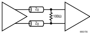
**Figure 35. Far-End Transmission Line Termination ( $Z_0 = 50\Omega$ )**
