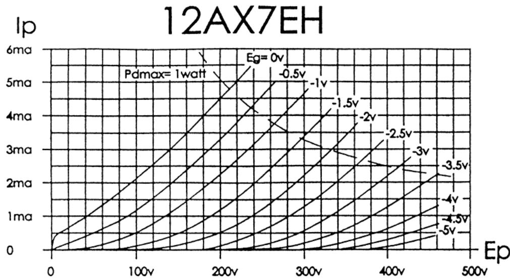
The 12AX7EH is a dual high mu triode with a spiral filament and special construction to minimize microphonic behavior. Ideal for replacement use in guitar amps and any place low noise and high gain is important.
