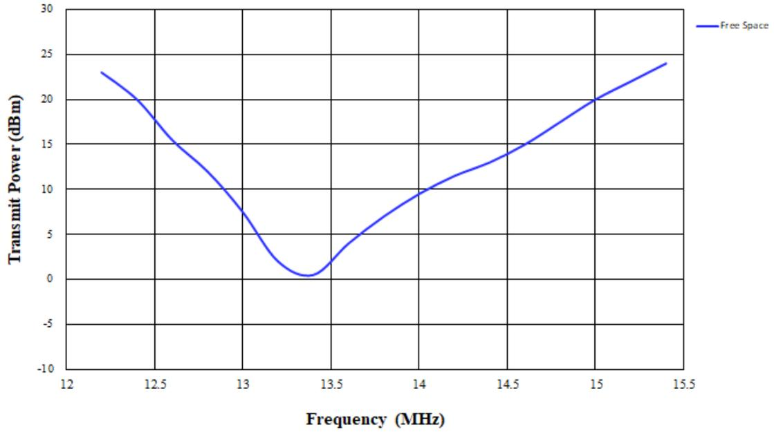
\*HF sensitivity shown in the figure is measured by Voyantic Tagformance HF Loop Antenna C60. Actual sensitivity performance is subject to the environment in practice.
