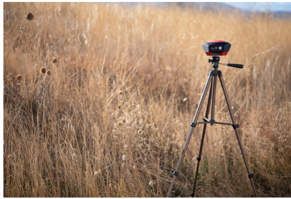
Temporary RTK Facet Base setup
