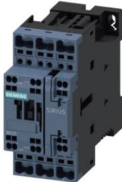
Power contactor, AC-3 25 A, 11 kW / 400 V 2 NO + 2 NC 24 V DC 4-pole size S0 Spring-type terminals 1 NO + 1 NC integrated
