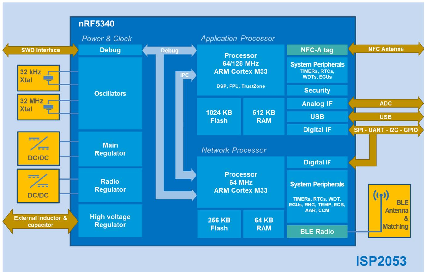
The application processor has 1 MB Flash, 512 KB RAM, a floating-point unit (FPU), an 8 KB 2-way associative cache and DSP instruction capabilities. The network processor is optimized for low power and offers 256 KB Flash and 64 KB RAM. In term of security, the Arm TrustZone provides trusted execution, the Arm CryptoCell-312 provides hardware-accelerated cryptography together with a root-of-trust and secure key storage management.
