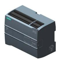
SIMATIC S7-1200F, CPU 1215 FC, compact CPU, DC/DC/relay, 2 PROFINET ports, onboard I/O: 14 DI 24 V DC; 10 DO relay 2 A, 2 AI 0-10 V DC, 2 AO 0-20 mA DC, Power supply: DC 20.4-28.8 V DC, Program/data memory 150 KB
