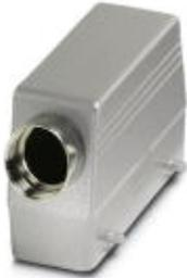
HEAVYCON sleeve housing B24, for double locking latch, height 76 mm, with support 1x M25, lateral conductor exit
