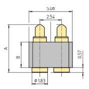
Replace NNN by number of poles, standard number of contact 2 to 20contacts See table below for final ordering number according to height and working range specifications
