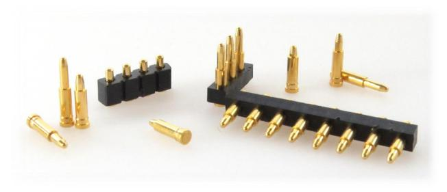
This new line of products have been designed to fit with most of applications, length of the contact is adaptive according your working range from 4.5 mm up to 8.5 mm. Base diameter is only 1.83 mm which allows to implant it with pitch of 0.1' (2.54mm).
