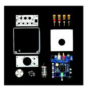
All electronic parts are preassembled to the PCB so that users just need a screwdriver and longnose pliers for assembly.
