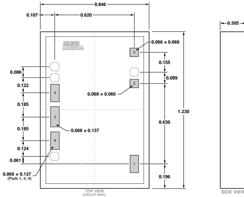
Figure 51. 6-Pad Bare Die [CHIP]
