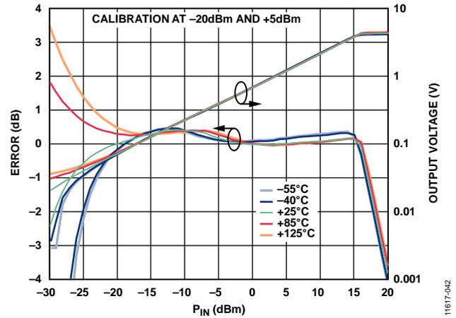
Figure 42. Conformance Error and Output Voltage vs. RF Input Power (P<sub>IN</sub>) for Various Temperatures (-55°C, -40°C, +25°C, +85°C, and +125°C) at 10 GHz Using Two Point Calibration
