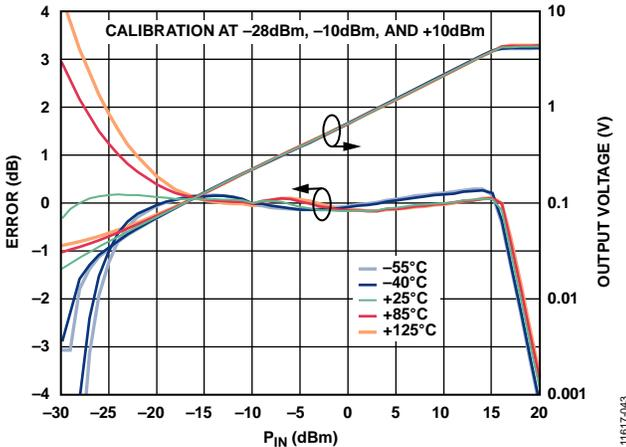
Figure 43. Conformance Error and Output Voltage vs. RF Input Power ( $P_{IN}$ ) and Temperature ( $-55^{\circ}\text{C}$ ,  $-40^{\circ}\text{C}$ ,  $+25^{\circ}\text{C}$ ,  $+85^{\circ}\text{C}$ ,  $+125^{\circ}\text{C}$ ) at 10 GHz Using Three Point Calibration
