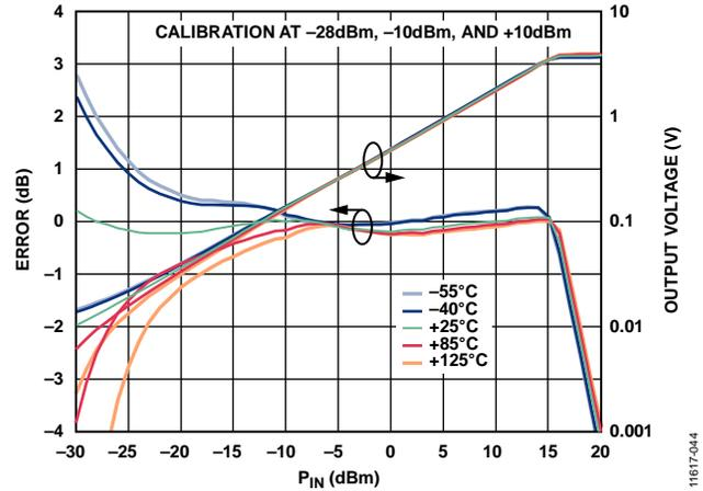
Figure 44. 10 GHz Conformance Error and Output Voltage vs. RF Input Power ( $P_{IN}$ ) for Second Device at  $+25^{\circ}\text{C}$ ,  $-40^{\circ}\text{C}$ ,  $-55^{\circ}\text{C}$ ,  $+85^{\circ}\text{C}$ , and  $+125^{\circ}\text{C}$
