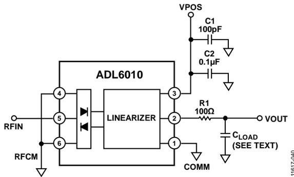
Figure 40. Basic Connections
