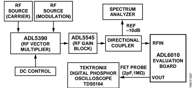
Figure 39. Hardware Configuration for Envelope Output Response Measurement
