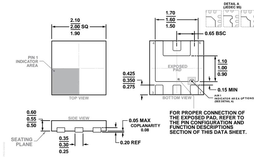
Figure 50. 6-Lead Lead Frame Chip Scale Package [LFCSPP]
